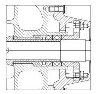
Cooled stuffing box with internal barrier fluid for pumping of clean liquids in suction operation or at inlet pressures up to 4 bar.
